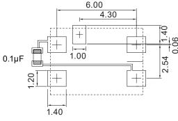
To ensure optimal oscillator performance, place a by-pass capacitor of 0.1uF as close to the part as possible between Vcc and GND PAD
