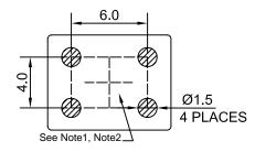
Note1: Copper in this area should be kept to a minimum to reduce heat loss from OCXO.
