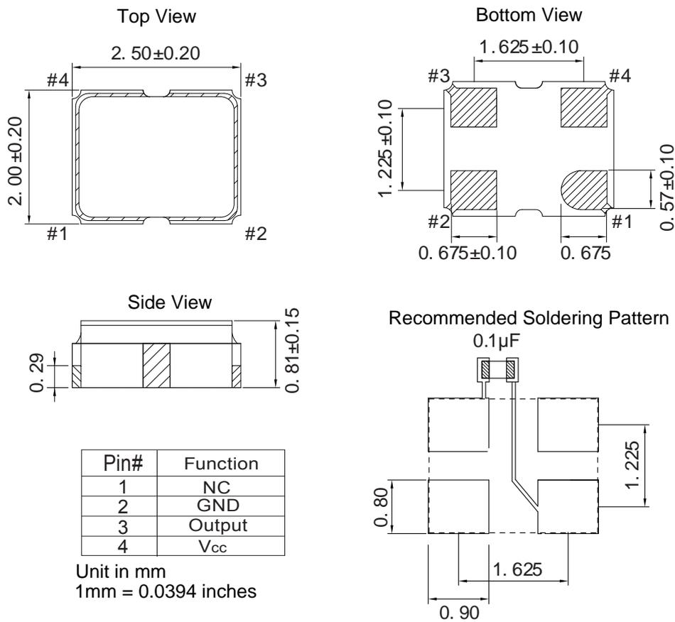
To ensure optimal oscillator performance, place a by-pass capacitor of 0.1uF as close to the part as possible between Vcc and GND PAD
