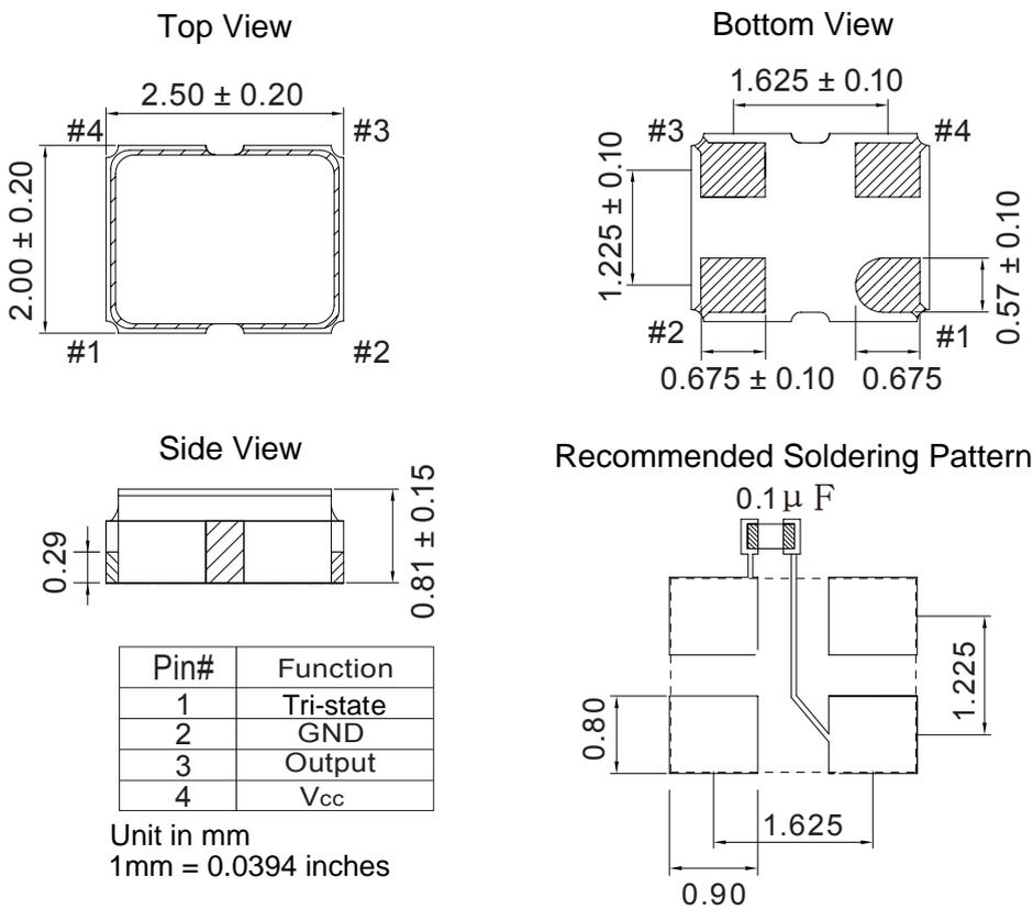
To ensure optimal oscillator performance, place a by-pass capacitor of 0.1 $\mu$ F as close to the part as possible between V<sub>CC</sub> and GND PAD
